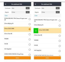
Click **Pre defined** to enter **Common Coordinate** interface, and then users are able to add a new coordinate system by clicking **Select**. Slide right and click the green button to check the coordinate system information.
