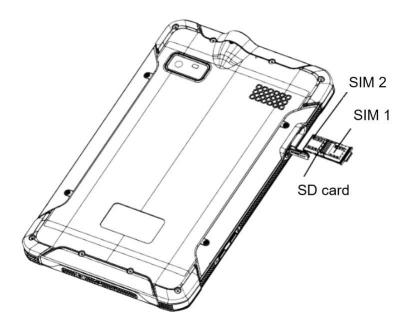
Please insert the SIM card and the MicroSD card in the direction of the diagram.
