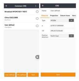
Set the right parameters according to the surveying area, and then click Save to finish CRS configuration.
